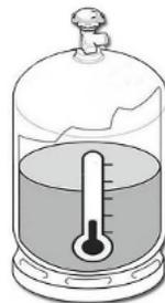
CONTINUOUS USE CAUSES CYLINDER TO FROST
